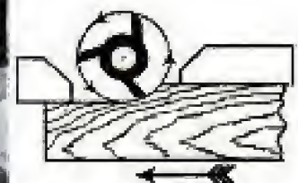
THIRD—MAKE A CUT. REPEAT CUT IF NEEDED
